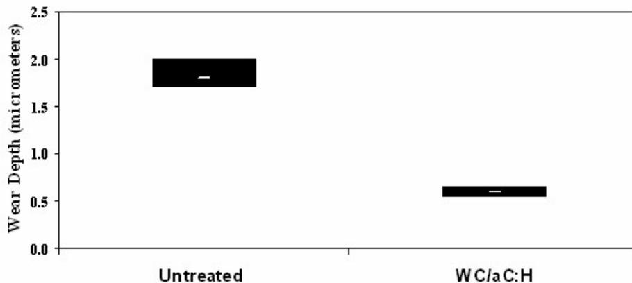
**Figure 6:** Results of laboratory testing for false brinelling in tapered roller bearings with untreated and WC/aC:H coated rollers. The data are expressed in terms of average wear depth with standard deviation. WC/aC:H coatings on the rollers changed the wear mode of the cup race from adhesive to mildly abrasive through the micro-polishing effect.
