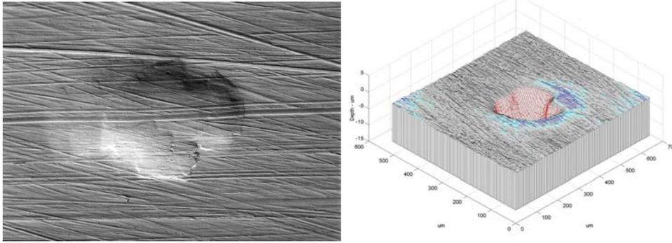
**Figure 9:** Magnified image of dent caused by metallic debris particle on raceway (left), and digitized image showing raised shoulders surrounding the dent (right).
