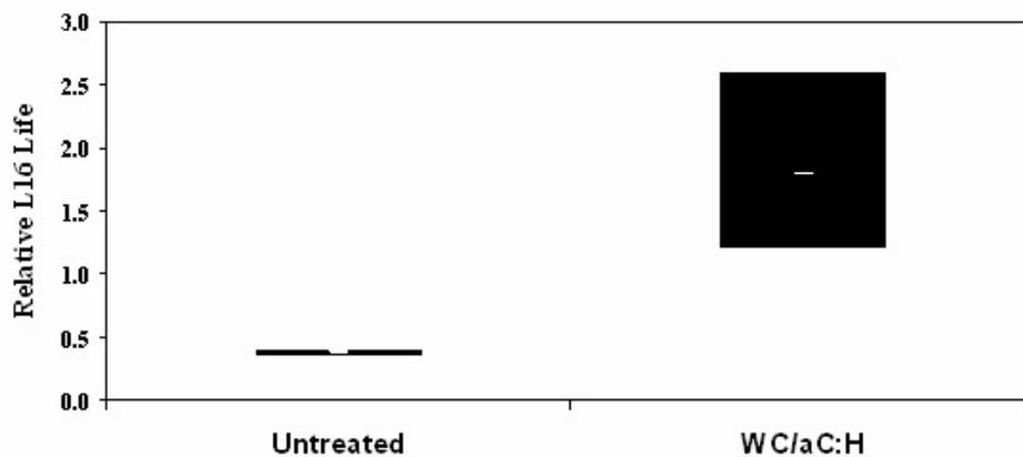
**Figure 5:** Results of laboratory testing showing the resistance to bearing life reduction caused by metallic debris provided by WC/aC:H coatings on rollers of tapered roller bearings.
