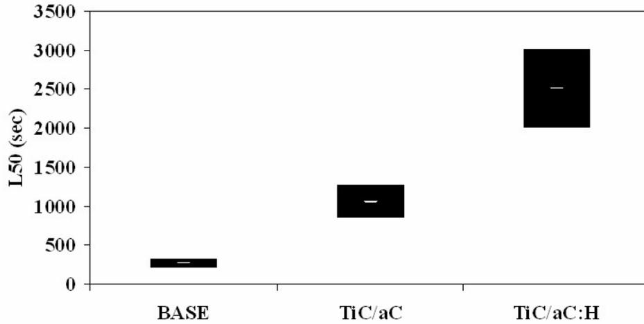
**Figure 4:**  $L_{50}$  time to rib-roller end failure of tapered roller bearings with and without coated roller ends. Tests were performed with an applied thrust load of 4448 N at a speed of 2700 rpm in a condition that mimics a loss of lubrication.
