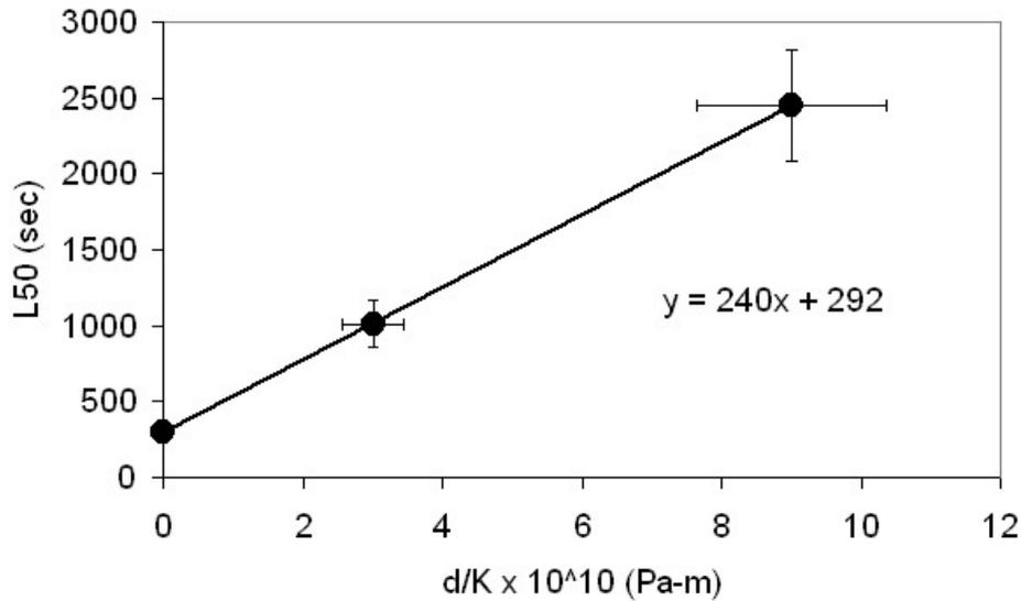
**Figure 8:** Data from Figure 4 plotted versus  $d/K$  for the bearings with uncoated roller ends ( $d/K = 0$ ), TiC/aC coated roller ends ( $d/K = 3 \times 10^{10}$  Pa-m), and TiC/aC:H coated roller ends ( $d/K = 9 \times 10^{10}$  Pa-m). The line is not a fit, but a calculation from Eq. 6.
