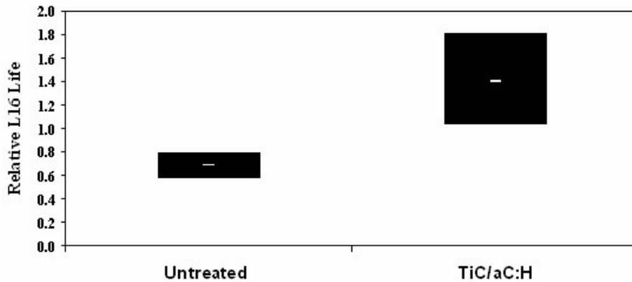
**Figure 3:** The  $L_{16}$  fatigue lives (normalized to the  $a_\lambda = 1$  calculated bearing life) of tapered roller bearings operating in  $\lambda \sim 0.6$  boundary layer lubrication with and without TiC/aC:H coatings on the rollers.
