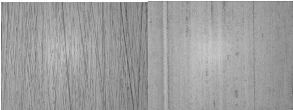
**Figure 7:** Optical images of cup raceways before (left) and after (right) being run against TiC/aC:H coated rollers in the fatigue life testing shown in Figure 3.
