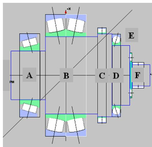
**Figure 1:** The basic types of rolling contact bearings are A – tapered roller, B – spherical, C – cylindrical, D – ball, E – needle thrust, and F – needle.
