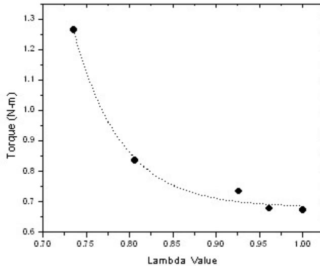
**Figure 10:** Measured torque of a tapered roller bearing as a function of  $\lambda$  (circles), and a fit to the data from Eq. 7.
