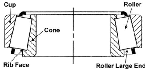
**Figure 2:** Cross sectional schematic showing the elements of a tapered roller bearing. Whereas rolling contact exists at the roller/cup and cone races, mostly sliding exists at the roller large end/rib face contact.
