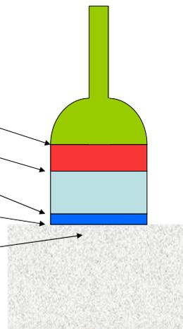
According to ASTM D4541, measurement is valid only if <50% of failure is due to glue.
