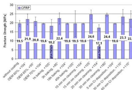
Conclusions: In most cases there is a cohesive failure of the substrate
