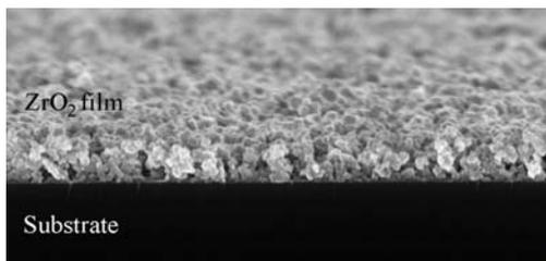
*Figure 1* Deposited zirconium oxide , containing nanoparticles.
