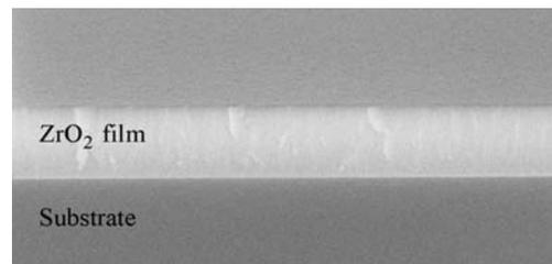
*Figure 2* Deposited smooth zirconium oxide film.
