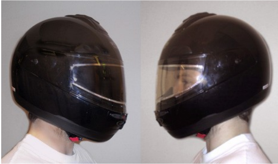
Fig. 6. Electrochromic visor for a motorcycle helmet in colored and bleached states.
