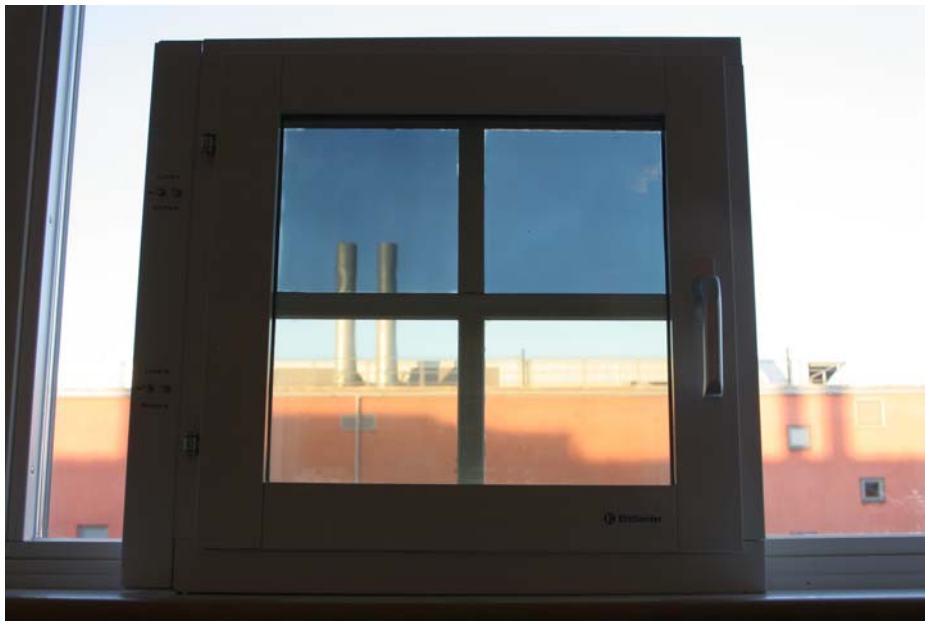
Fig. 7. "Smart window" prototype with four 30 x 30 cm 2 panels.
