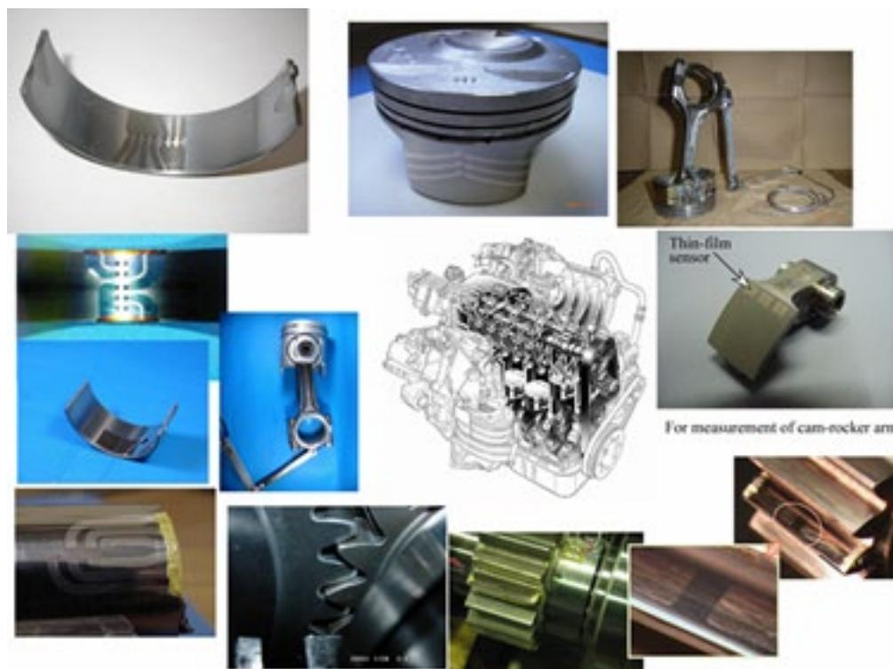
FIGURE 1. Application of thin-film sensors for engine parts and machinery (Engine main bearings, Connecting rod bearings, Piston skirts, piston pin-boss, Spur and helical gears, etc..)
